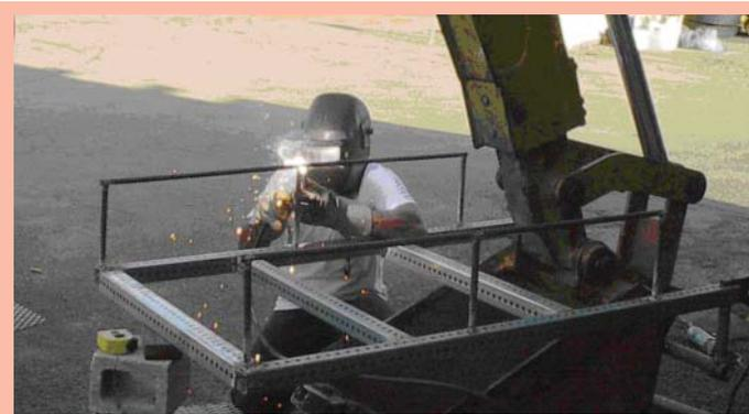
**Lionel Haili Jr.** welding the rebar for the siderail of the wire mesh basket.
