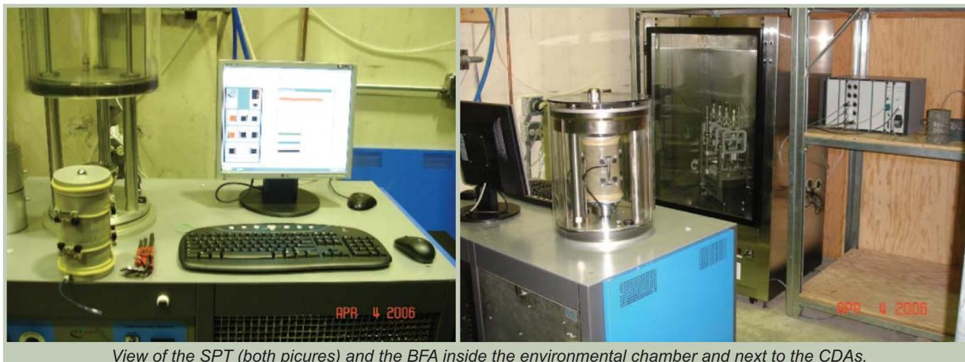
View of the SPT (both pictures) and the BFA inside the environmental chamber and next to the CDAs.
