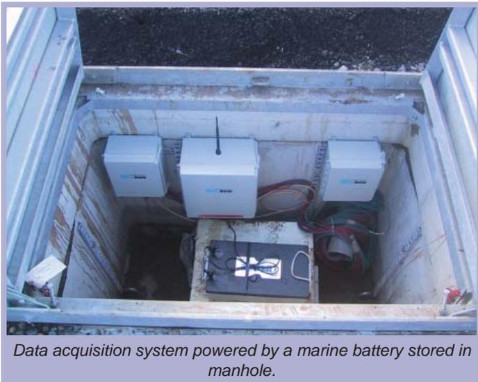
*Data acquisition system powered by a marine battery stored in manhole.*
