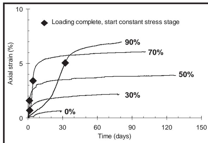
Preliminary results are shown for the Manoa clay in the bottom figure. They indicate, as expected, that creep increases with deviatoric stress intensity. As of this date creep tests have only been conducted on the Manoa clay and the Kapolei red silt. It appears that the finer-grained Manoa clay is more creep-susceptible due to its higher Atterberg limits. Also, the Manoa clay undergoes significant strength gain with time. The testing of all soils is expected to be completed in January 2001.
