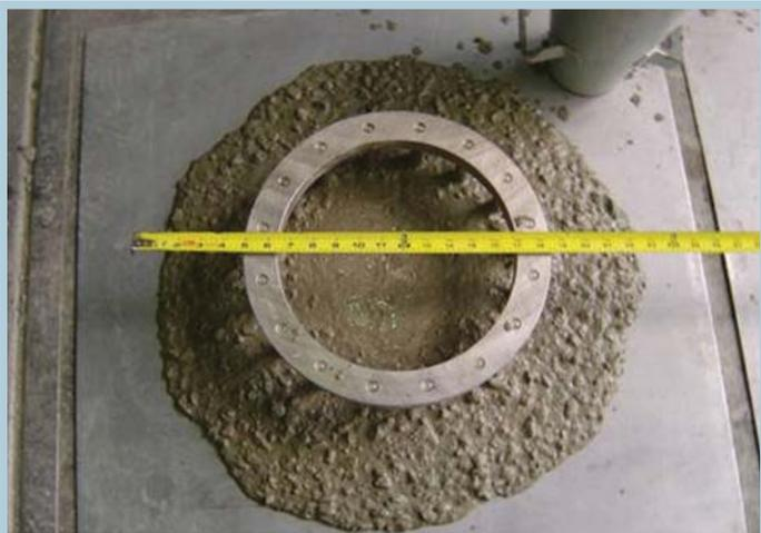
*J-ring flow test on SCC mixture*
