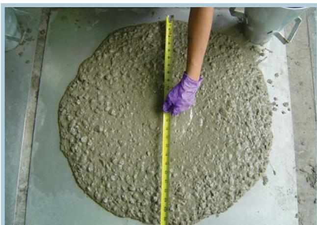
Typical slump flow test
