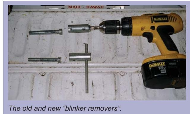
The second device invented by Edwin replaced a crude manual tool that came with the blinker barricades to remove the housing for changing batteries. It was a steel rod attached to a socket that couldn't be turned more than 90 degrees and perhaps causing "carpal tunnel disease for workers," Edwin muses.
