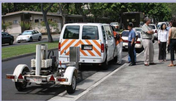
*HDOT's Falling Weight Deflectometer (FWD)*
